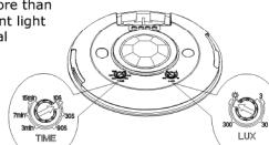
**NOTE:** when testing in daylight, please turn LUX knob to (SUN) position, otherwise the sensor lamp could not work! If the lamp is more than 60W, the distance between lamp and sensor should be 60cm at least.
