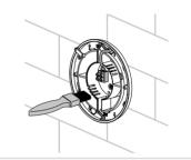
Install the front panel to the fan. Screw in the fixing screw. Connect power supply.
