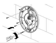
Connect the fan to the electric mains according to the connections diagram. Install the front panel by turning it clockwise. Thread the fixing screw.
