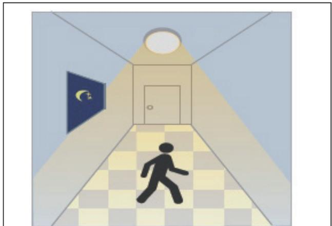
When motion is detected, and the daylight is insufficient, the light will be ON.
