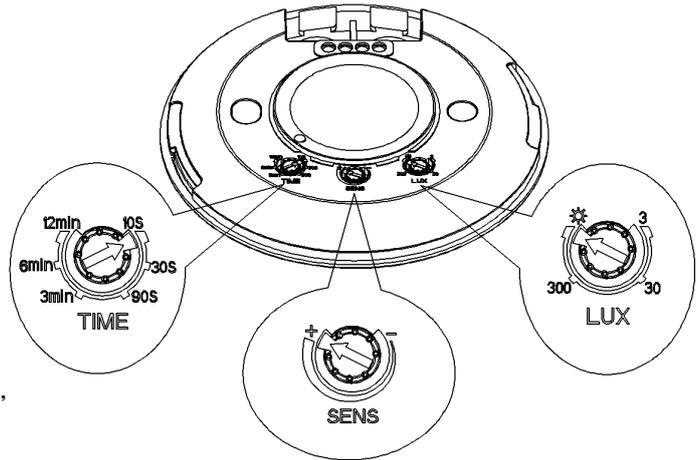
**Note: when testing in daylight, please turn LUX knob to ☀ (SUN) position, otherwise the sensor lamp could not work!**
