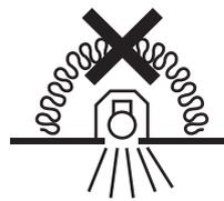
Luminaires not suitable for covering with thermally insulating material.
