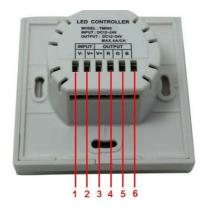
"1", "2": power input pins, input voltage range is 12-24V, "1" is negative pole, and "2" is positive pole.
