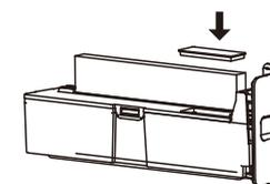
7. Push the tank back into the purifier.
