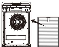
B. There are differences between the inside and the outside of the absorption filter 2 (Cellular -Activated Carbon Filter and cold catalyst filter). Attention: The side with a handle should be placed outwards
