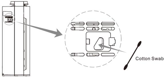
Wipe the lens with a dry cotton swab periodically to remove any dirt. (Moisture or tobacco smoke residue may cause it to no longer work properly). First remove the particulate sensor cover, use a dry cotton swab to wipe the lens.
