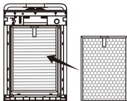
C. There are differences between the inside and the outside of the front filter (pre-filter). Attention: The side with a handle should be placed outwards
