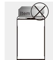
5. Do not block the exhaust vent or supply vent. For example, do not place an object on top of the exhaust vent or in front of the supply vent.
