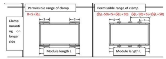
Figure 4 Position requirements of connecting points
