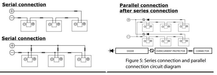
The number of modules in series connection in each strand shall be calculated as per requirements. The open circuit voltage value under the expected lowest temperature shall not exceed the maximum system voltage value stipulated for modules (V-TAC module maximum system voltage is DC1500V according to IEC61730) and other values required by DC electric parts.
