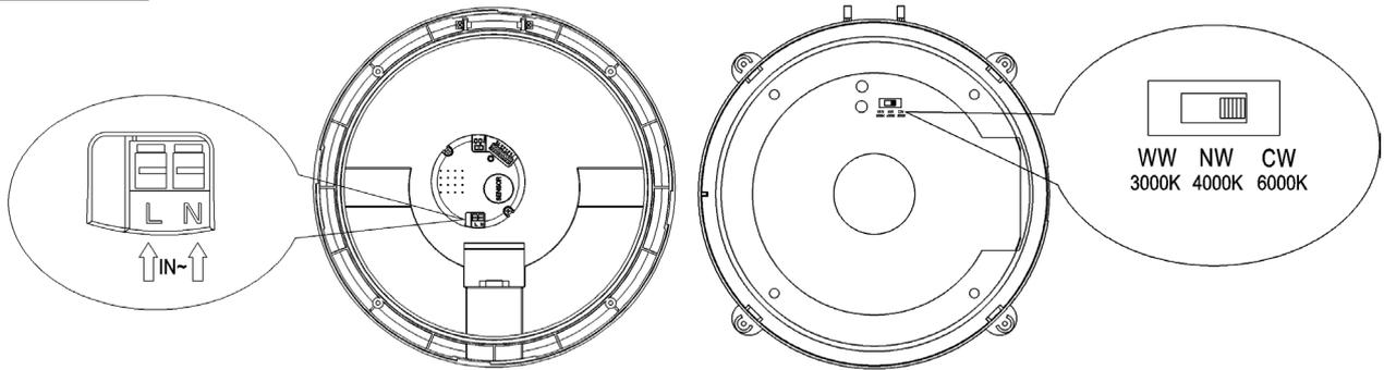
Remarks: you can slide the switch to adjust the color temperature to 3000K, 4000K or 6000K
