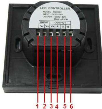
“1”, “2”: power input pins, input voltage range is 12-24V, “1” is negative pole, and “2” is positive pole.
